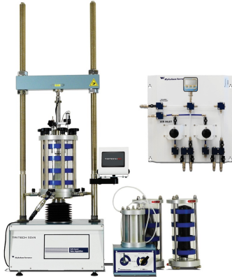
Standard triaxial system with built-in data acquisition and air/water interface pressure system
